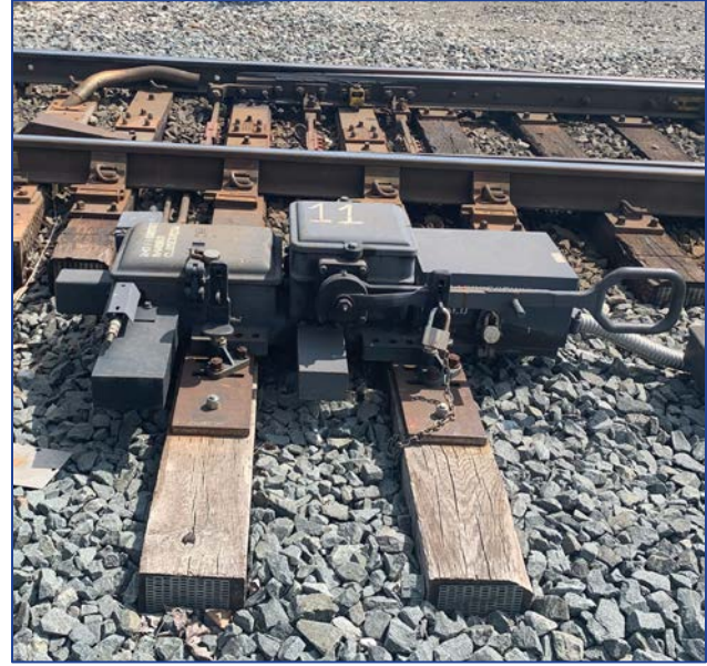
Powered rail switch with switch heater at Pullman Junction (will replace manually operated switches)
