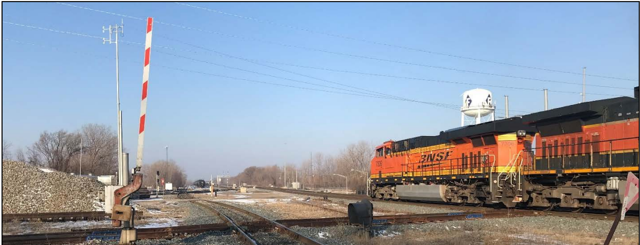
Existing gate at the crossing of the CRL/SCIH Main Track and the NS Verson Lead Track. Each time a train travels through the crossing on the north-south tracks, the conductor must dismount to manually raise and then lower the gate arm located on the east-west tracks. EW3A will replace this gate with modern railroad signals which will indicate safe crossing to all trains.
